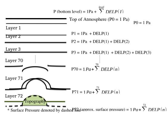
Figure 2. Diagram showing how pressure levels are calculated for vertical fields in OMUFPMET and OMVFPMET.
